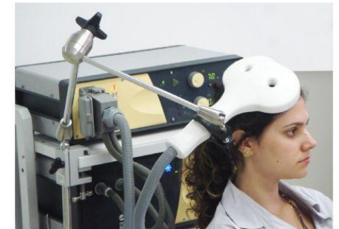
Figure 6.28 Running current through a magnetic coil generates an electric field via induction (top), which can activate or inactivate neural circuits in TMS (bottom).
