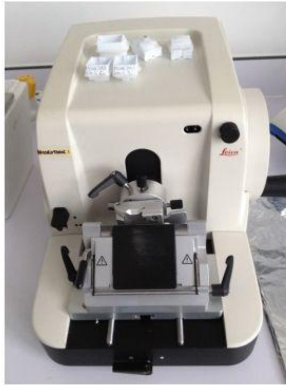
Figure 6.21 A microtome (left) or a cryostat (right) are devices for taking brain sections. The microtome fits on a tabletop, and cuts accurately down to 100 \mu\text{M} thin. The cryostat is larger, and can cut 10 \mu\text{M} thin slices.
